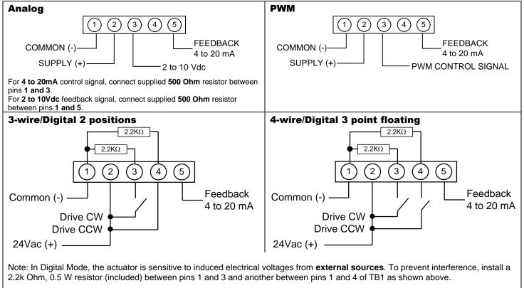
Note: In any of the above wiring configurations, connect a supplied **500 Ohm** resistor between pins **1** and **5** for a 2-10Vdc feedback signal.
