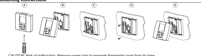
CAUTION: Risk of malfunction. Remove power prior to separate thermostat cover from its base.
