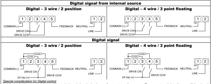
In this mode, the actuator is sensitive to induced electrical voltages **from external sources**. To prevent such interference, if the signal on pins 4 and 3 on TB1 are from an **external 24 Vac source**, install a resistor 2.2kOhm, 0.5W between pins 4 and 1 and another 2.2kOhms, 0.5W between pins 3 and 1 of TB1. These resistors are included.
