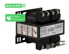
Transformer, Type T, industrial control, 100 VA, 240/480 VAC primary / 120 VAC secondary, 1 phase, 50/60 Hz, 55 °C rise
