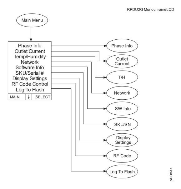
**NOTE:** The display screen is restricted to four lines per page. If there are more than four available selections, they will appear on multiple pages. "Outlet Current" only appears on Metered-by-Outlet and Metered-by-Outlet with Switching units. "Temp/Humidity" only appears when an AP9335T or AP9335TH sensor is attached.
