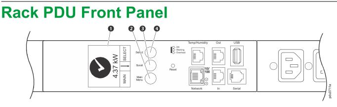
**NOTE:** Your Rack PDU is configured so the display backlight turns off after 10 minutes of inactivity. The backlight can be turned on by depressing any button below the display.
