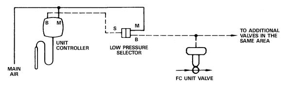
Figure-4 Low Pressure Selector Relay (2372-351) used as Booster Relay.
