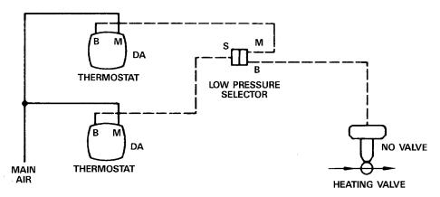
Figure-3 2372-351 Low Pressure Selector Relay.
