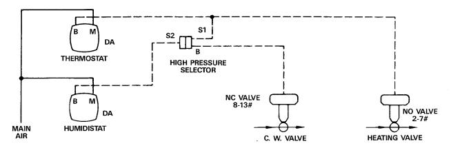
Figure-2 2372-352 High Pressure Selector Relay.
