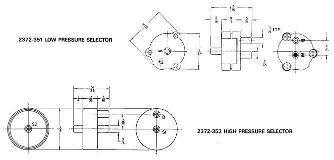
Figure-1 Mounting Dimensions.
