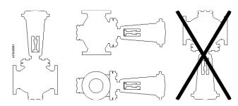
Figure 1. Acceptable Mounting Positions.
