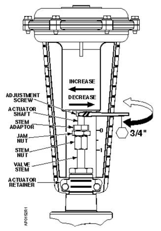
Figure 15. Spring Adjustment.
