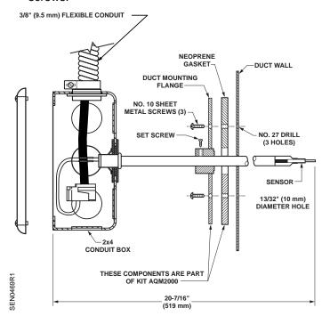
Figure 1. Duct Point Sensor Installation.
