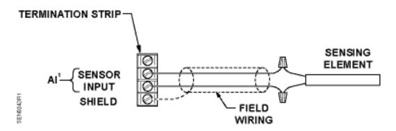
1. Configure the analog input (AI) point for sensor input.
