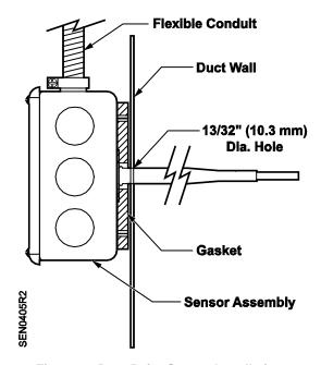
Figure 1. Duct Point Sensor Installation.
