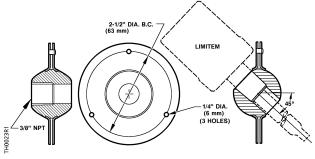
Figure 2. Swivel Flange Mounting Kit Part Number 356-090.
