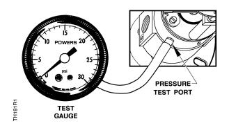
Figure 9. Using the Pressure Test Port.
