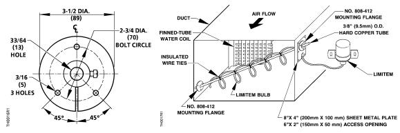
Figure 7. Installation of TH 357 Averaging Bulb in a Duct.
