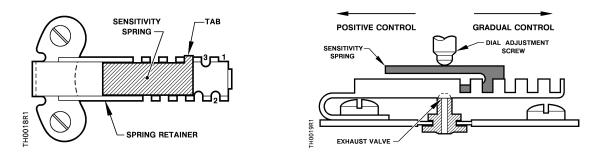
Figure 10. Sensitivity Spring Setting.
