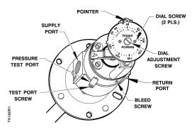
Figure 8. LIMITEM<sup>®</sup> Cover Removed.
