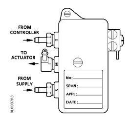
Figure 3. Mounting Relay Ports.
