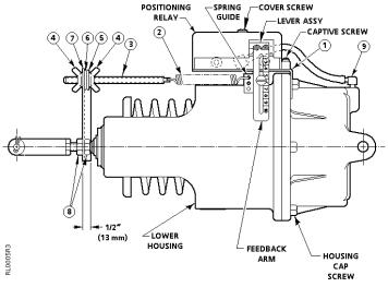
Figure 1. Positioning Relay Mounting Kit 147-276 on the No. 6 Damper Actuator.
