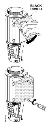
Figure 8. Attaching the cover.
