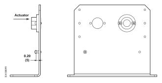
Figure 1. Anti-rotation Screw Location.
