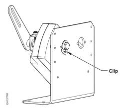
Figure 3. Clip Position for Lever above the Actuator.
