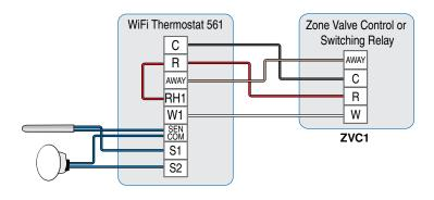
The WiFi Thermostat 561 operates a baseboard/radiator using an air temperature sensor. The air temperature sensor can be either built-in and/or external.
