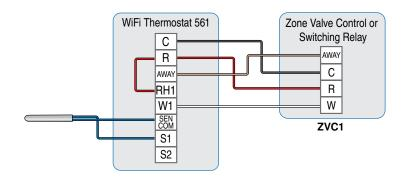
The WiFi Thermostat 561 operates a radiant floor heating system. The thermostat uses both air and floor temperature sensors. The air temperature sensor can be either built-in and/or external.
