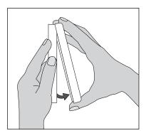
While holding the base section in one hand, pull the lower half of the display front towards you to pivot it away from the base.
