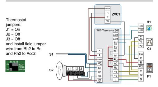
The WiFi Thermostat 563 operates a first stage radiant floor and a two-stage air-to-air heat pump for heating, cooling, and dehumidification, a backup electric heater, and a humidifier.
