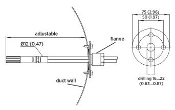
Left: Installation kit for duct mounting. Right: Installation flange. Aluminum or stainless steel.
