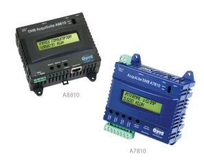
The A7810 AcquiLite™ and A8810 AcquiSuite™ data acquisition server for embedded applications allows users to collect energy data from meters and environmental sensors and send it via Modbus
