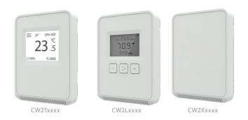
The CW2 Series of air quality sensors for living space is a flexible multi-sensor platform for use with BAS controllers designed to accept 4 to 20mA, 0 to 5Vdc or 0 to 10Vdc outputs. CW2 Series sensors are available with three user interface options: touchscreen, LCD with three buttons and blank. CO<sub>2</sub> and temperature sensors are included with all CW2 Series air quality sensors. Models with VOC sensors and relative humidity sensors are also available.
