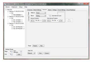
Use this tab to set up the demand sub-internal duration and the sub-interval counter. This tab also allows the user to reset these values using the Reset button. The Present Demand and Max Demand values can be reset using the buttons at the right.
