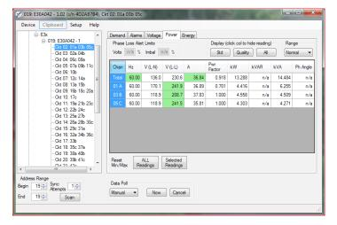
This tab allows the user to view all real-time data values for a single Logical Meter. The table shows the channels of the selected Logical Meter in the left most column. The other columns show the readings for each parameter. Use the Filter button to reduce the number of parameters visible, if desired.
