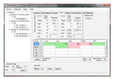
This tab is used to configure the alarm thresholds. This tab is also divided into sections.
