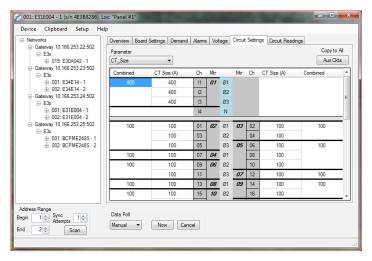
The table that appears below the Parameters field shows all circuits. For solid-core (E30) models, the CT sizes are fixed at 100 A. For split-core (E31) models, the fields in the Combined and CT Size columns are editable and can be set to 50 A, 100 A or 200
