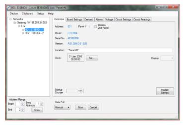
This tab shows identification information for the selected panel. The Location field is editable. Enter a relevant description for the panel's location.
