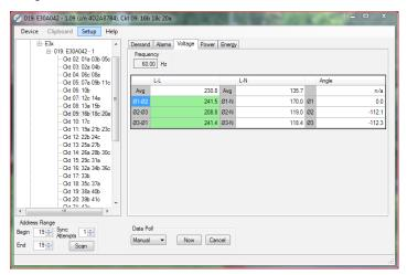
This tab allows the user to view the line-line and line neutral voltages and the phase angles for each Logical Meter in real time. This tab is display-only, with no editable fields. Since all Logical Meters share the same voltage connection, all of them will read the same Voltage values.
