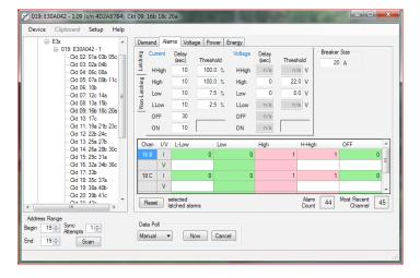
Alarms are defined previously in this document, in the Configure the Meter section. Use this tab to view alarm states and reset latching alarms for the selected Logical Meter. Note that there are separate sub-tabs along the left edge of the pane for latching and non-latching alarms.
