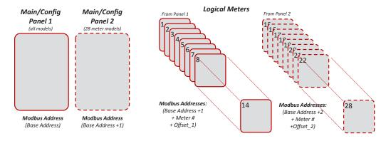
All measurement data can be accessed through the two Main/Configuration panels (at base address and base address + 1), however an alternate method of accessing the data can be used to simplify integration, especially in applications that are not monitoring full panelboards. This alternate method, referred to as "Logical Meter by Address" is enabled by default on E34x models and disabled on all others. It can be enabled or disabled on any E3x model (see "1. Overview tab" below).
