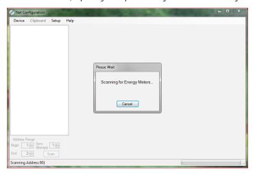
5. You can use the Scan All Networks Button to locate all meters on all networks, but the Modbus addresses scanned should be set first for each network (default for each network is 1-16).
