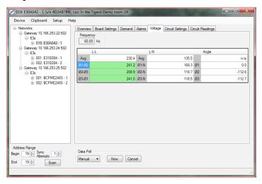
This tab allows the user to view the frequency, line-line and line-neutral voltages, and the phase angles in real time. This tab is display-only, with no editable fields.
