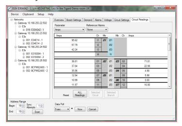
This tab shows the most recent data for any measurement selected. Use the drop-down list in the Parameter and Reference/ Alarms fields to select what values to view. The table below repopulates with the data values selected, according to the option selected in the Data Polling section.
