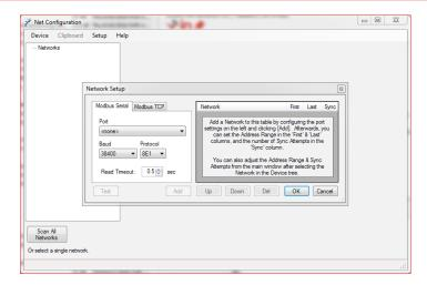
2. Modbus TCP: If configuring an E3xE model, enter the IP address for the meter. Otherwise, enter the IP address of the Modbus gateway. Read timeout is user selectable from 0.1 sec to 10 sec.
