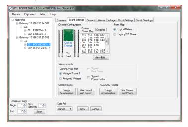
The Board Settings tab allows the user to configure the board. The tab is divided into sections.
