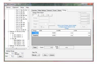
This tab allows the user for view the accumulated Energy value for a single Meter.
