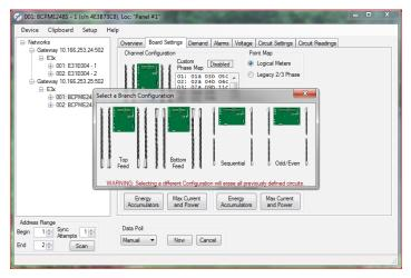
Below are the two Branch Configuration options available for E31 (split-core) and E34 models.
