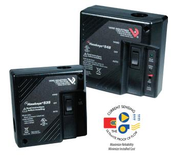
The Hawkeye 5xx Series combines an industrial grade load-switching relay, current status switch\*, and Hand-Off-Auto (HOA) switch\* in an easy-to-install remote enclosure, making the series ideal for monitoring, directly controlling, and troubleshooting the control wiring of fractional horsepower motors.
