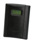
HW Series deluxe humidity transmitters provide an ideal solution for measuring relative humidity in all conditions. All devices are equipped with a thin-film capacitive sensor that is easily replaceable in the field. These sensors are calibrated to NIST standards, with certificates available (see Ordering Information; choose "N" in NIST block). Temperature sensing options are also available.
