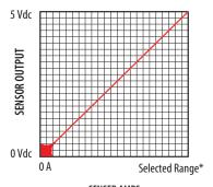
SENSED AMPS \*Factory calibrated ranges selected with the amperage range switch
