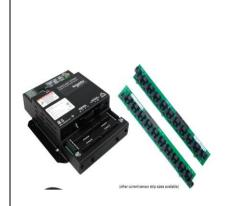
**The E30 series** consists of a data acquisition board and up to 4x 21-unit current sensor strips, with 8x auxiliary inputs. The strips are mounted on each side of the panel board along the termination points of each breaker. The conductor passes through the appropriate current sensor before terminating at the breaker. Each strip transmits the current data to the data acquisition board.
