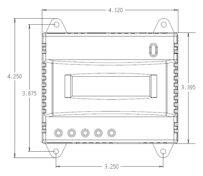
The AcquiLite has 4 mounting holes for use with a #6 screw. The drawing above shows the relative position of the mounting holes.
