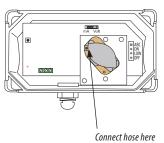
2. Start flowing nitrogen gas (0 ppm CO<sub>3</sub>). Use a flow rate of 0.3 to 0.5 liter/minute.
