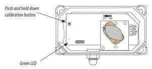
4. Continue flowing gas through the sensor until the LED deluminates. Estimated calibration time is 5 minutes. Remove the hose from the calibration port when complete.
