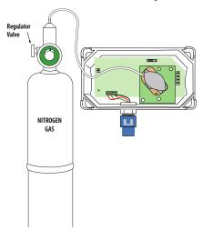
3. Push and hold down the calibration button until the LED illuminates.
