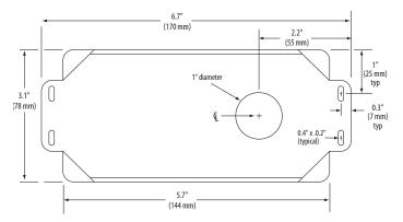
3. Insert the probe into the hole. Rotate the housing so that the widest surface is perpendicular to the air flow.
