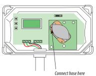
2. Start flowing nitrogen gas (0 ppm CO<sub>3</sub>). Use a flow rate of 0.3 to 0.5 liter/minute.
