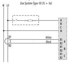
Diagram 2: 1-Phase Line-to-Line 2-Wire System 1 CT
