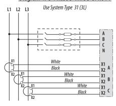
Diagram 5: 3-Phase 4-Wire Wye Direct Voltage Input
