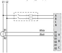
Diagram 3: 1-Phase Direct Voltage Connection 2 CT
