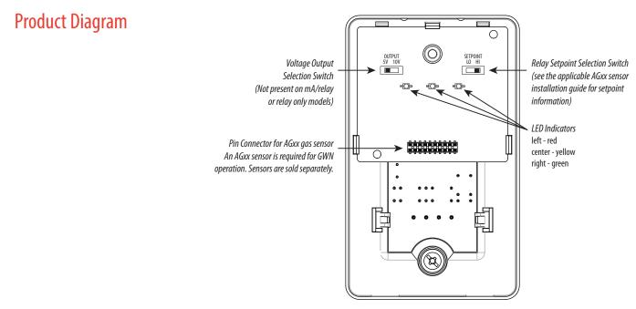
The voltage output selection switch is only available on voltage output models. For mA/relay output and relay only models, this space is empty.
