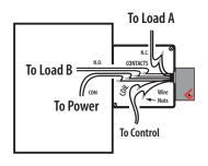
\* Isolate any unused wires, e.g. wire nut.
